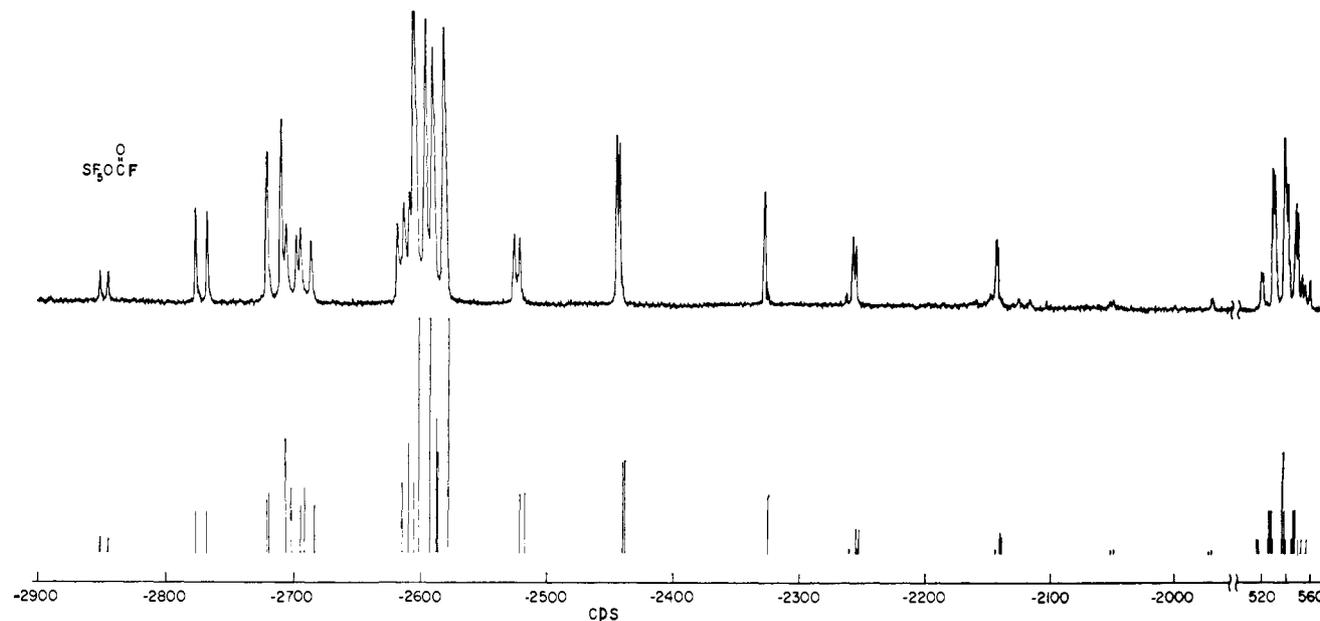
Figure 6. Nuclear magnetic resonance spectrum of pentafluorosulfur fluoroformate taken at 40 Mc. Peaks between  $-2900$  and  $-2550$  cps are due to the  $\text{SF}_4$  fluorine atoms. Peaks between  $-2550$  and  $-1950$  cps are due to the unique fluorine atom on sulfur. Peaks in the vicinity of  $+540$  cps are due to the fluorine atom bonded to carbon.
