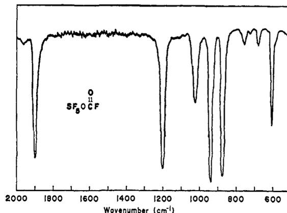
Figure 4. Infrared spectrum of pentafluorosulfur fluoroformate (3 mm).
