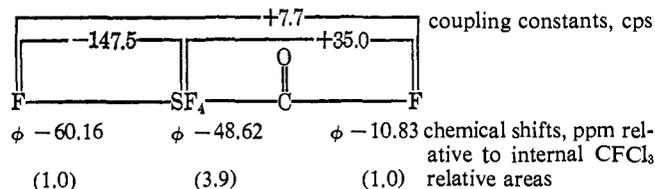
Figure 2. Nuclear magnetic resonance data calculated for  $\text{SF}_5\text{C}(\text{O})\text{F}$ . The signs of the coupling constants are relative to one another and not necessarily absolute.
