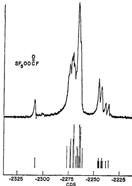
Figure 8. Nuclear magnetic resonance spectrum of the  $\text{SF}_5$  region of pentafluorosulfur peroxoformate taken at 40 Mc.
