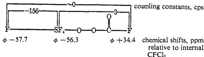
Figure 9. Nuclear magnetic resonance data calculated for  $\text{SF}_5\text{OOC(O)F}$ .
