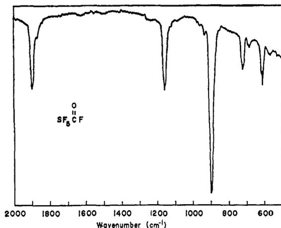
Figure 1. Infrared spectrum of pentafluorosulfur carbonyl fluoride (2 mm).
