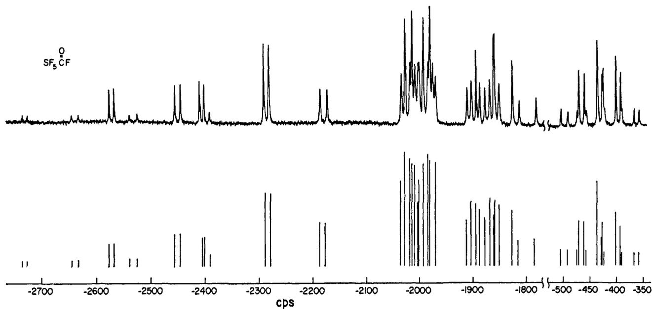
Figure 3. Nuclear magnetic resonance spectrum of pentafluorosulfur carbonyl fluoride taken at 40 Mc. Peaks between  $-2750$  and  $-2150$  cps are due to the unique fluorine atom on sulfur. Peaks between  $-2050$  and  $1750$  cps are due to the  $\text{SF}_4$  fluorine atoms, and peaks between  $-520$  and  $-350$  cps are due to the fluorine atom bonded to carbon.
