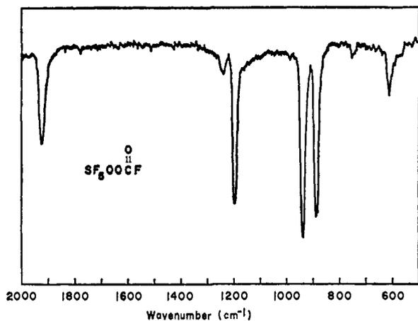
Figure 7. Infrared spectrum of pentafluorosulfur peroxoformate (2 mm).
